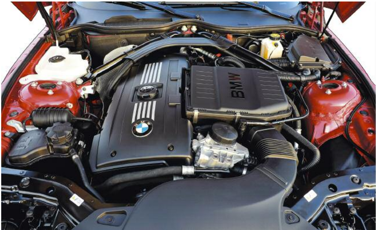
View of the Z4 sDrive35is engine compartment with N54B30T0 engine
